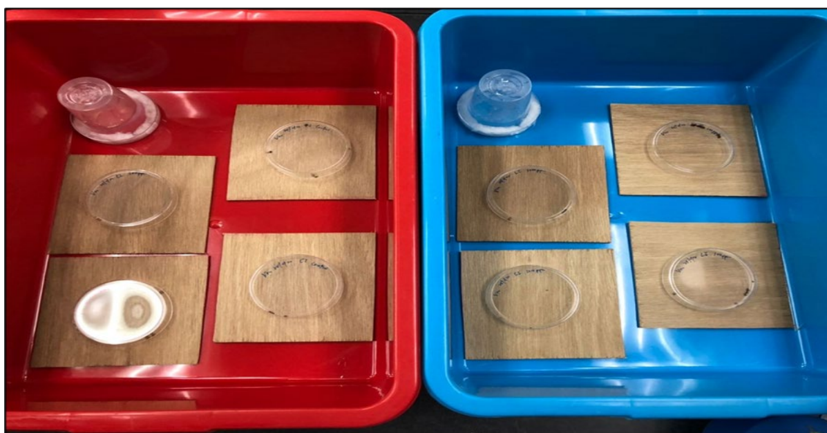
Figure 1. The setting of insecticide bioassay. The treated surfaces were placed in the basins, where the moisture level and temperature were regulated optimally. Bed bugs were confined inside the Petri dishes
