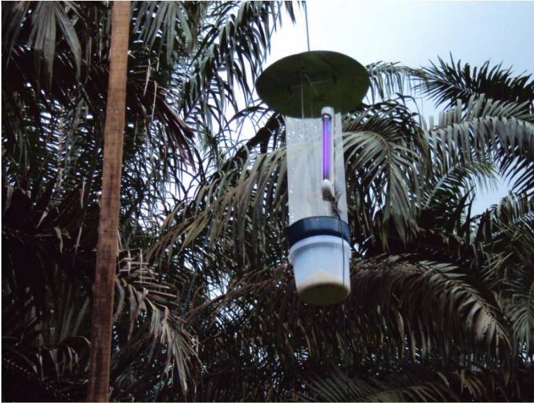
Figure 1. Canopy-height Light Trap.
