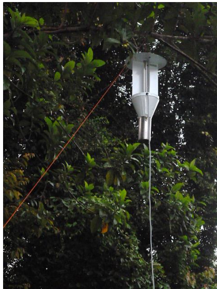
Figure 2 Light trap with florescent and UV light for insect sampling
