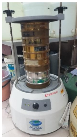
Plate 2. Mechanical shaker used in particle size analysis
