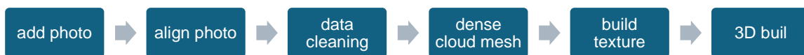
Figure 6. Stages in UAV image processing using Agisoft Metashape Professional software to produce orthophoto and 3D models
