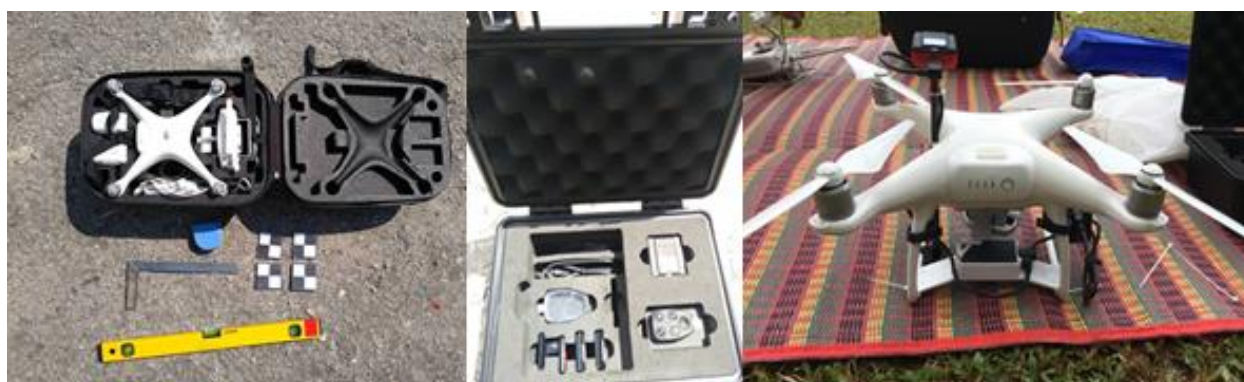
Figure 4. Parrot Sequoia Sensor mounting on DJI Phantom 4.
