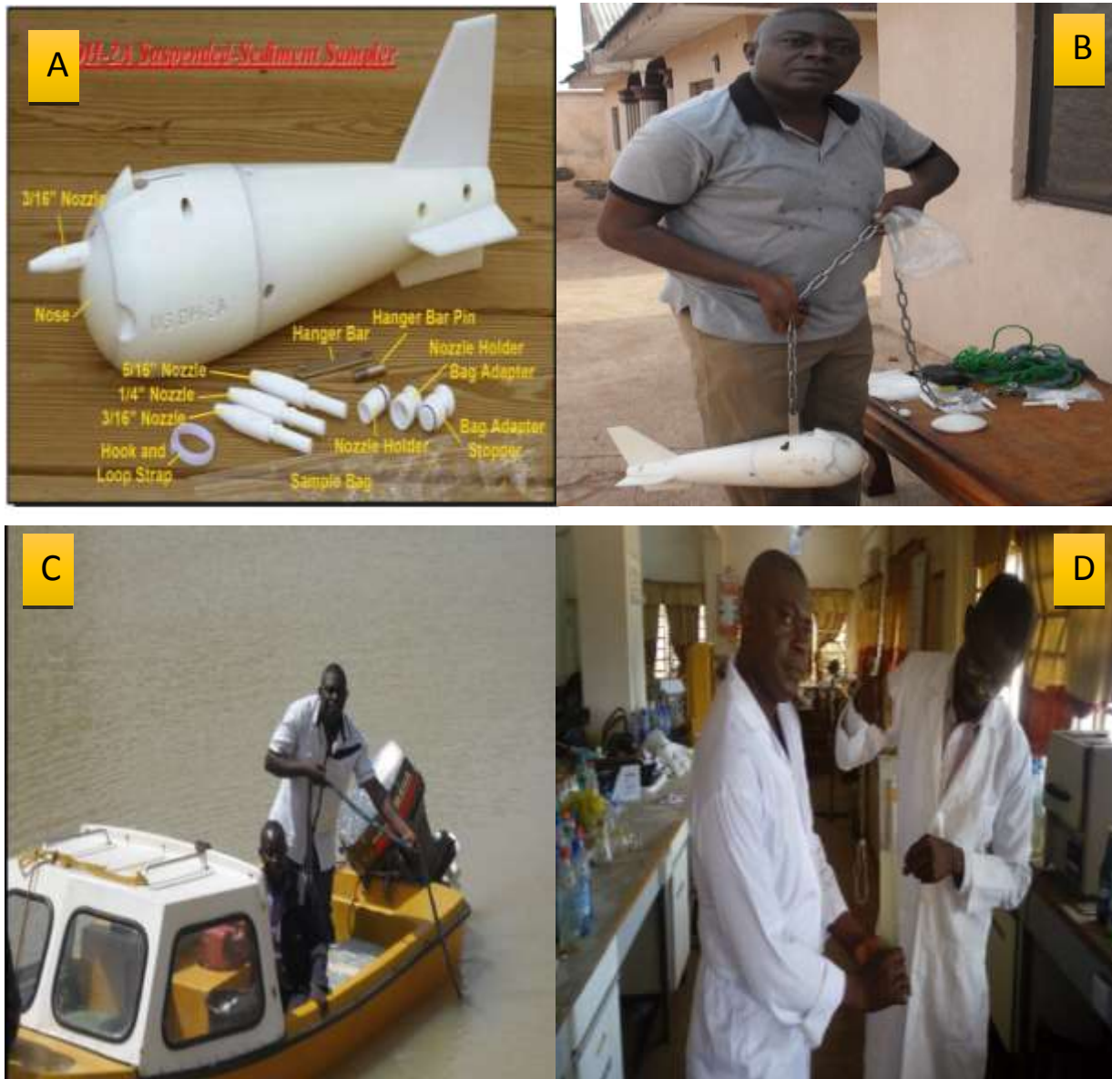
Figure 1. A) US-DH-2A sampler, B) US-DH-2A sampler assemblage, C) Water samples collections at sampling points, D) Laboratory analysis of SSC and Turbidity.
